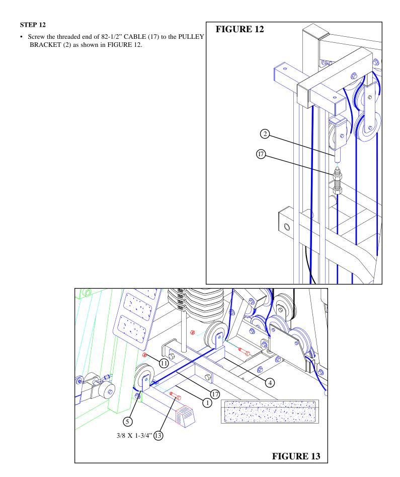
Attach one 3-1/2" PULLEY (5) to the FRONT LEG (1) and one 3-1/2" PULLEY (5) to the BASE CONNECTION (4) using two 3/8 X 1-3/4" BOLTS (13) and two 3/8" LOCKNUTS (11). (Note: Make sure CABLE (17) is running under PULLEYS.)
